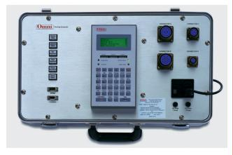
The Omni 3000 Portable Prover Computer (PPC) is a light-weight, suitcase-mounted proving computer. It has the ability to control the entire prove sequence, including control of four-way valves of a bi-directional prover. Illuminated LED switches give a clear indication of prove sequence status. All process and control signals are distributed amongst flow connectors (see technical specifications).
